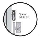
Note: do not install with hinge upside down, ie. with ball bearing and cap at bottom of hinge, this allows water to fill hinge barrel and can cause hinge seizure.
